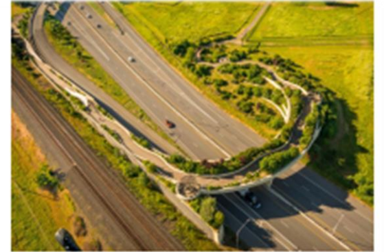
Vancouver Land Bridge (Vancouver, Canada) An earth-covered pedestrian bridge linking trail to parkland and waterfront
